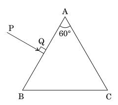
A ray PQ is incident normally on the face AB of a triangular prism of refracting angle of 60°, made of a transparent material of refractive index  $2/\sqrt{3}$ , as shown in the figure. Trace the path of the ray as it passes through the prism. Also calculate the angle of emergence and angle of deviation.
